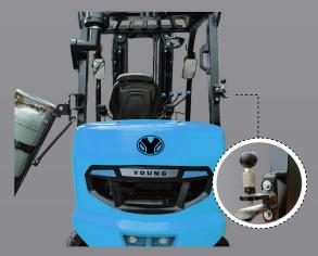
**Standard-equipped with swing down LPG tank bracket**, alloqing foreasy replacement of the fuel tank.
