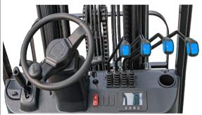
Utilization of a small-diameter steering wheel, electro-hydraulic gearshift, and ratchet type hand-brake, greatly enhancing driving comfort.
