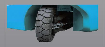
Integration of a high-angle cast steering axle to reduce the overall turning radius of the vehicle.
