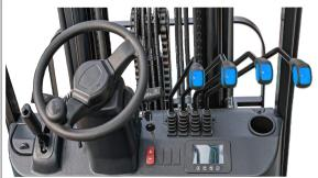
Utilization of a small-diameter steering wheel, electro-hydraulic gearshift, and ratchet type hand-brake, greatly enhancing driving comfort.
